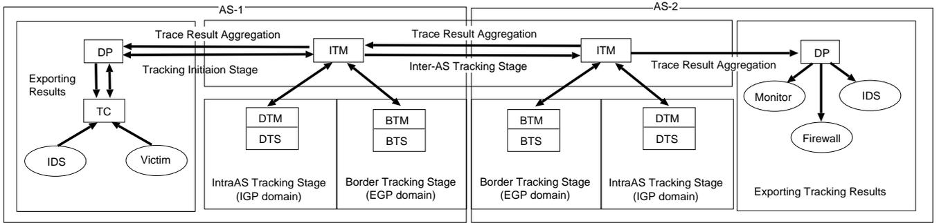
Figure 3: Procedures of an attack tracking on InterTrack
